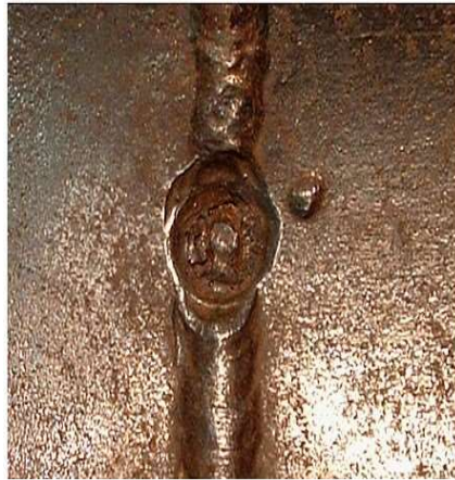
Figure 1: Weld Burn Through
