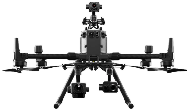
Figure 2: LiDAR Drone for outdoor (Photo courtesy DJI Zenmuse H20)
