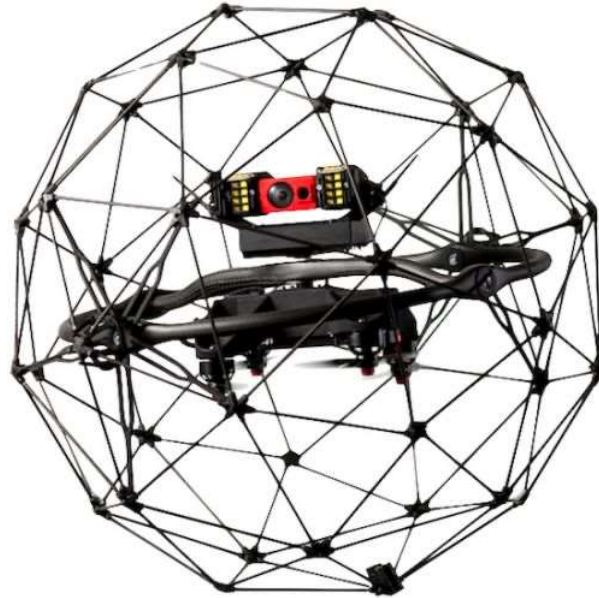
Figure 1: Collision resistant UAV chiefly used indoors (Photo courtesy- Flyability)
