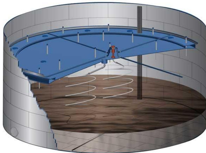
Figure 2: External Floating Roof Tank
