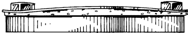
Figure 1: Illustration of a Flange Bending or Bowing
