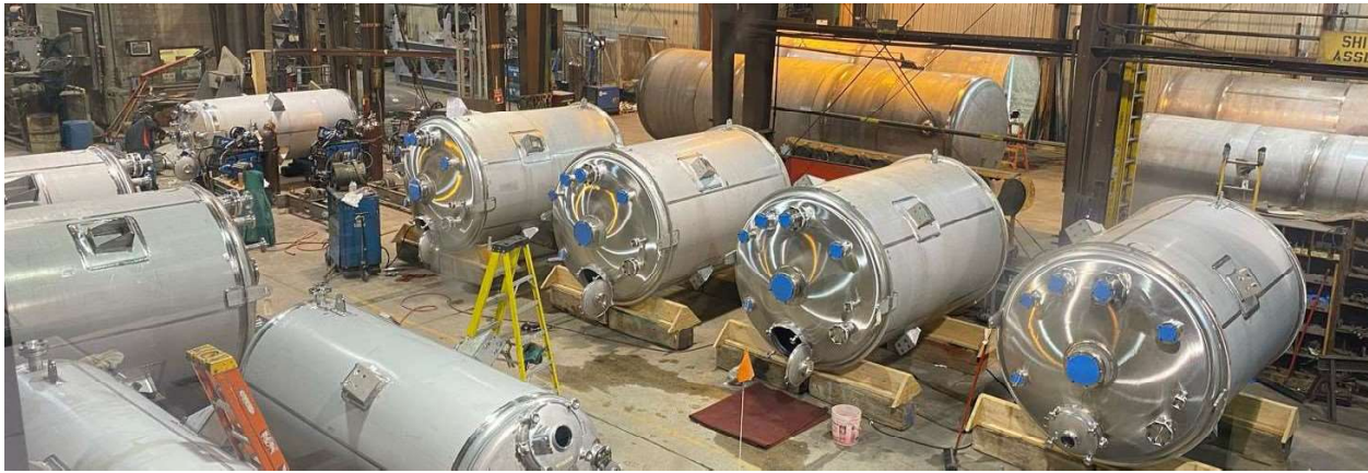
Figure 1: Pressure Vessels after Completion of Hydrostatic Tests
