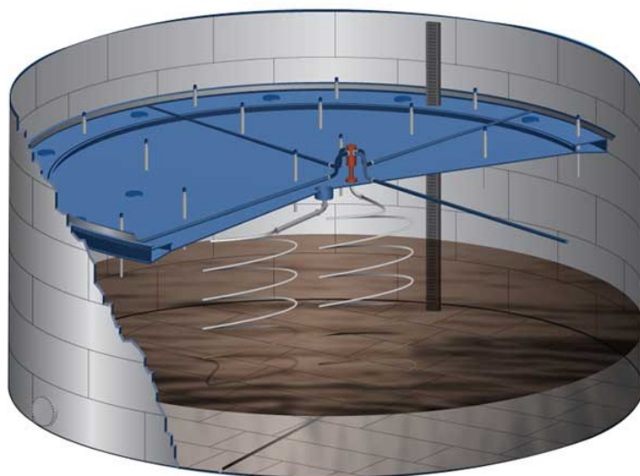
Figure 2: External Floating Roof Tank
