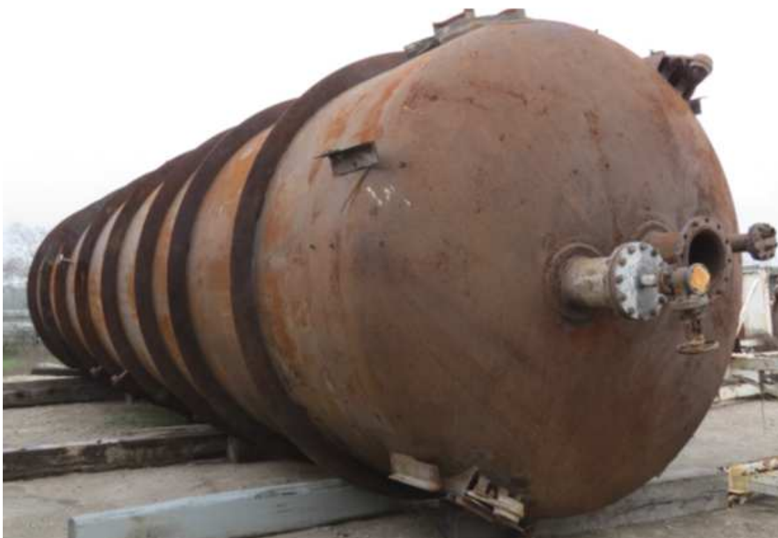
Figure 1. A vacuum tower made of SA-285C from the 1950's. Shell Martinez serial #C-4201
