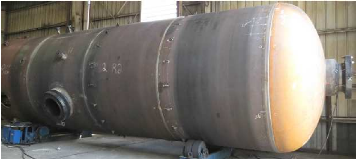
Figure 3. An example of a vertical drum made of SA-516-70
