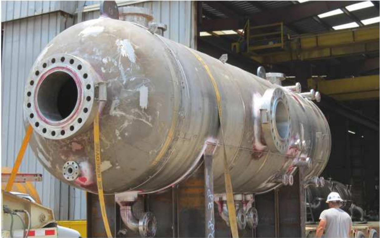
Figure 5. This 316 stainless separator is the first to be used offshore in place of a clad vessel
